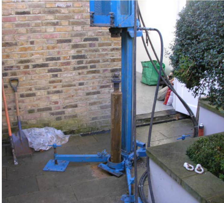
Figure 50. Restricted access modular site investigation rig
