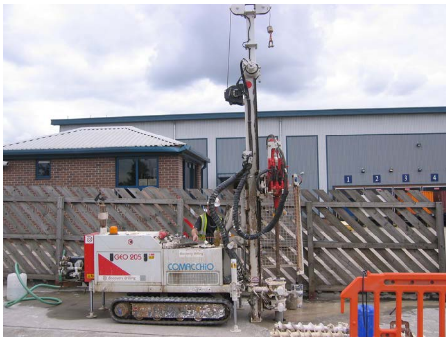
Figure 51. Full access site investigation drilling rig
